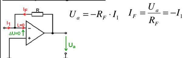
$$U_a = -R_F \cdot I_1 \quad I_F = \frac{U_a}{R_F} = -I_1$$
