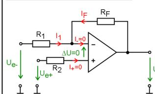
$$U_a = U_{e+} \cdot \left( \frac{R_F}{R_1} + 1 \right) - U_{e-} \cdot \frac{R_F}{R_1}$$
