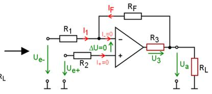
$$U_a = U_e + \left( \frac{R_F}{R_1} + 1 \right) \cdot U_e - \frac{R_F}{R_1} \cdot U_e \quad I_F = \frac{U_a - U_{e+}}{R_F} = -I_1 = \frac{U_{e+} - U_{e-}}{R_1}$$
