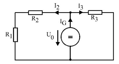
Werte:  $I_3 = 2A$ ,  $R_1 = 20\Omega$ ,  $R_2 = 60\Omega$ ,  $R_3 = 40\Omega$ ,
