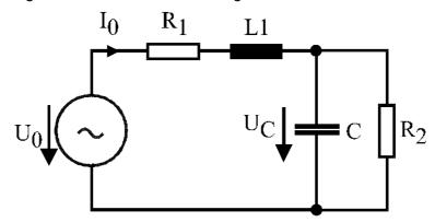
Werte:  $U_C = 10V$ ,  $R_1 = 20\Omega$ ,  $R_2 = 40\Omega$ ,  $L_1 = 64mH$ ,  $C = 128\mu F$ , f = 50Hz
