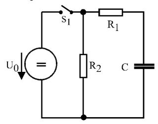
Werte:  $U_0 = 30V$ ,  $R_1 = 10k\Omega$ ,  $R_2 = 20k\Omega$ ,  $C = 100\mu F$
