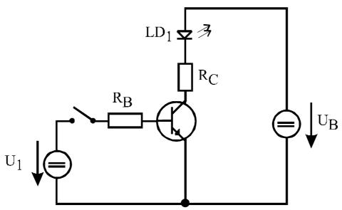
Werte:  $U_B = 4.5V$ ,  $U_1 = 10V$ ,  $R_C = 200\Omega$ ,  $R_B = 74.4k\Omega$
