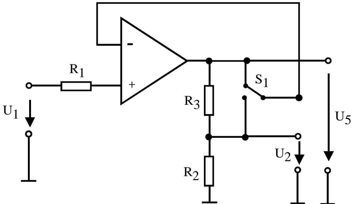
Werte:  $R_1 = 40\text{k}\Omega$ ,  $R_2 = 10\text{k}\Omega$ ,  $R_3 = 30\text{k}\Omega$ ,  $U_1 = 1\text{V}$
