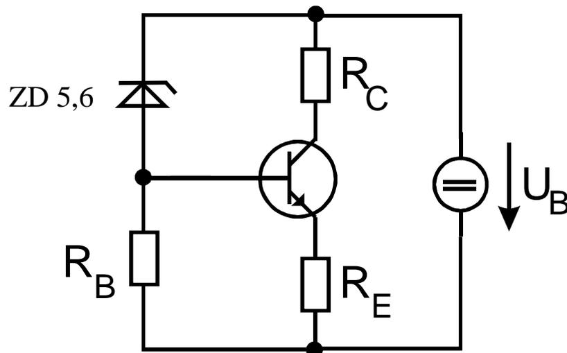
Werte:  $U_B = 9V$ ,  $R_B = 100\text{ k}\Omega$ ,  $R_C = R_E = 1\text{ k}\Omega$ ,  $B=200$
