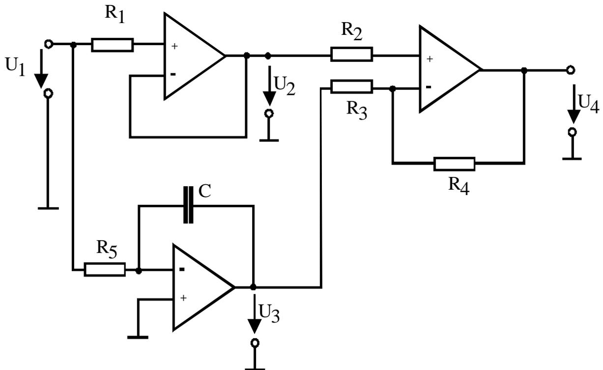
Werte:  $R_1 = 10\text{k}\Omega$ ,  $R_2 = 20\text{k}\Omega$ ,  $R_3 = 30\text{k}\Omega$ ,  $R_4 = 40\text{k}\Omega$ ,  $R_5 = 50\text{k}\Omega$ ,  $C = 20\text{nF}$
