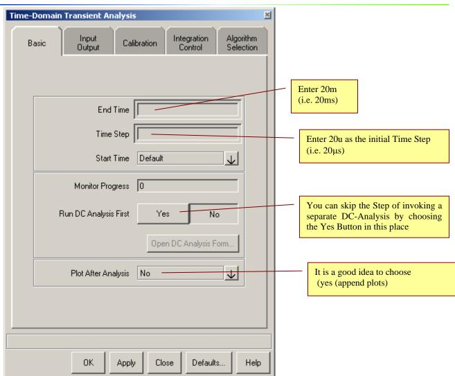
After doing the settings you can click the OK- Button and the Simulation will start. If the design is new or modified, you will be asked if the design should be saved before netlisting. Answer with 'yes'.
